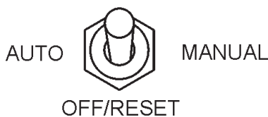
Figure 57. MPEC Control Switch (Off/Reset)
